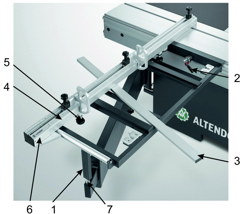
Fig. 5-13 Installing the cross-slide
