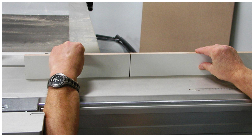
Fig. 5-42 Checking the 0° -setting
