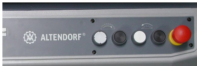
Fig. 6-19 Operating panel on the machine stand (model X/TE)
